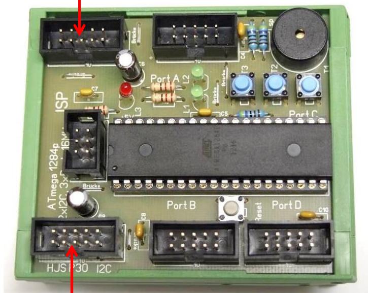
Board 1 (ATmega 1284p, 16MHz)
